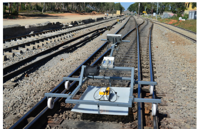
Fig. 1. Typical GPR survey at real track using 800 MHz antenna using specially designed wheel insulated trolley.
