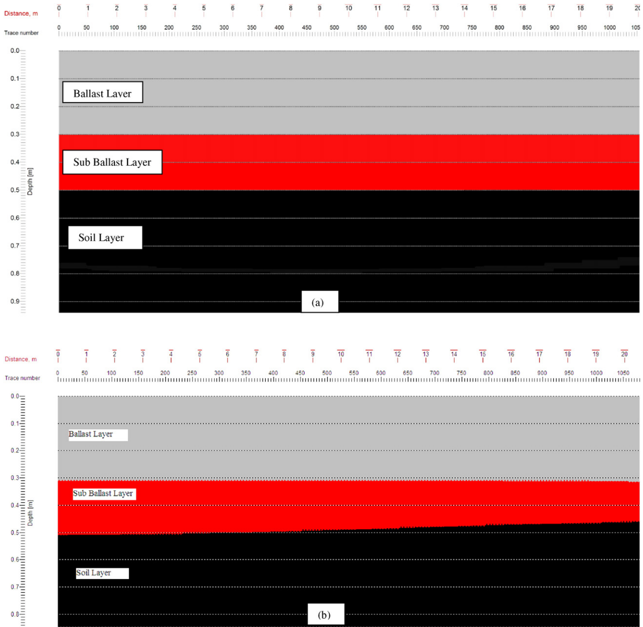
Fig. 3. Processed radargram of real railway track by applying the scattering amplitude envelope approach. (a) 500 MHz GPR antenna and (b) 800 MHz GPR antenna.
